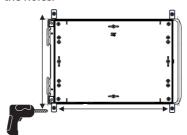
Screw the Yard Reader Station into place using fasteners suitable for the wall material. Fasteners are not included in the scope of delivery. Make sure that the screws are securely in place and that the Yard Reader Station is stable and secure.
