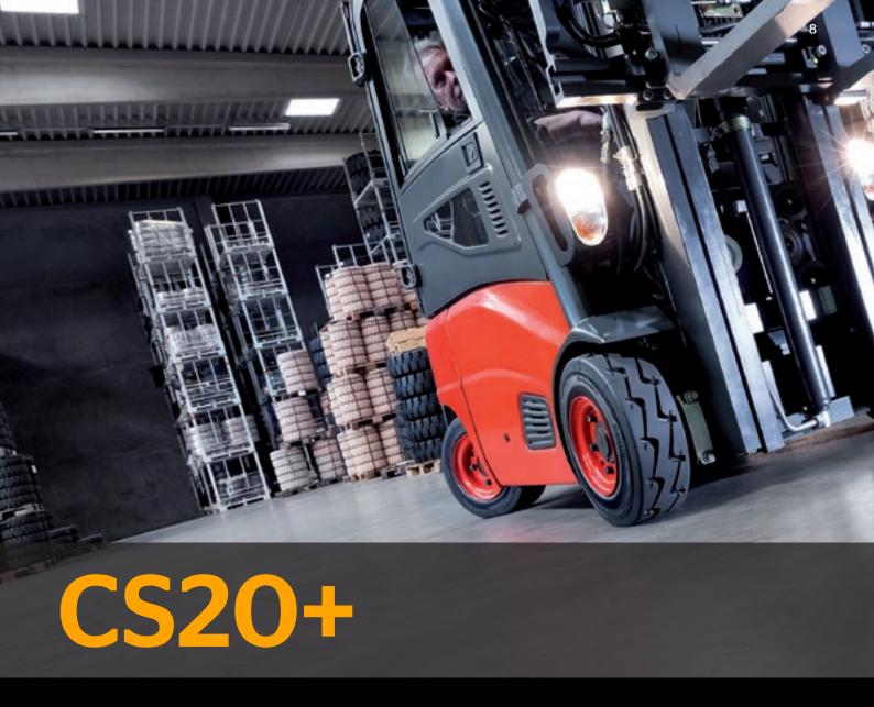
The CS20 has always been an extraordinary solid tyre. By means of the new Continental Plus Compound, it becomes even better in the shape of CS20+. Its unique double-L profile with closed shoulders ensures not only exceptionally precise steering and cornering, but also minimises vibration, resulting in excellent driving comfort.
