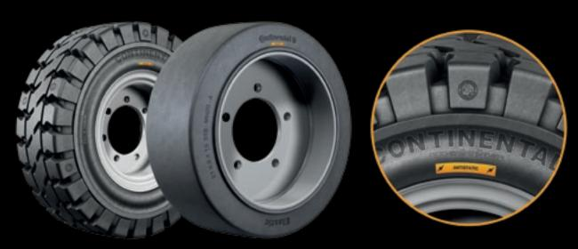
Every vehicle generates and stores electronic charge whilst driving as conventional tyres are practically non-conductive. normally this is not a problem, yet in certain sensitive application areas, uncontrolled electronic discharges may cause sparks. That is why we have developed antistatic versions of our Super Elastic Tyres SC20 and MH20, which prevent static charging.
